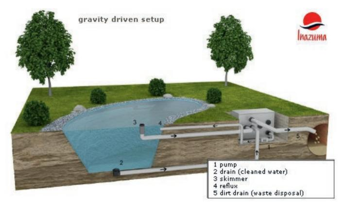
The filter must be attached to solid and plane ground. After positioning the filter, both axes (lengthwise and crosswise) must be aligned along the water-level. The use of a spirit level is heavily recommended.
