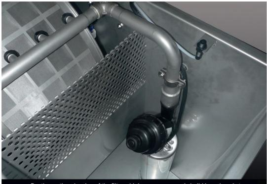
For the routine cleaning of the filter a high-pressure pump is build in and ready to use. It is made out of stainless steel. Constantly immersed it is frost-proof and low-noise.
