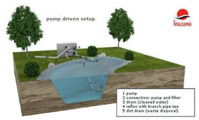
The filter must be attached to solid and plane ground. After positioning the filter, both axes (lengthwise and crosswise) must be aligned along the water-level. The use of a spirit level is heavily recommended.
