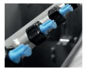
It is possible that one or more high-pressure nozzles get jammed. This leads to poorer results and shorter cleansing intervals.
